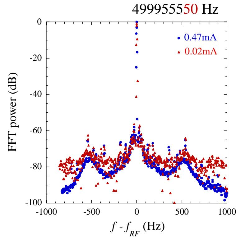
Current dependence of fs side-band.  $f_{RF}$  peak is normalized to 0dB. White noise is subtracted from the data at 0.02mA
