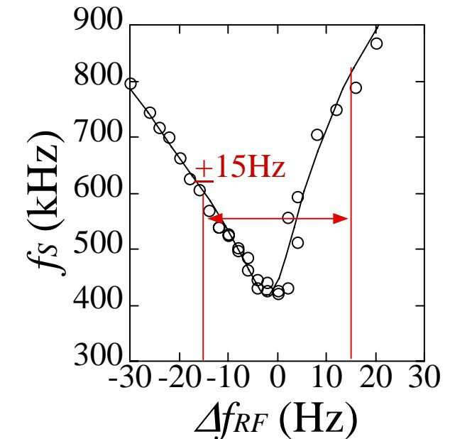
Synchrotron Oscillation is enhanced at  $\delta > 0$
