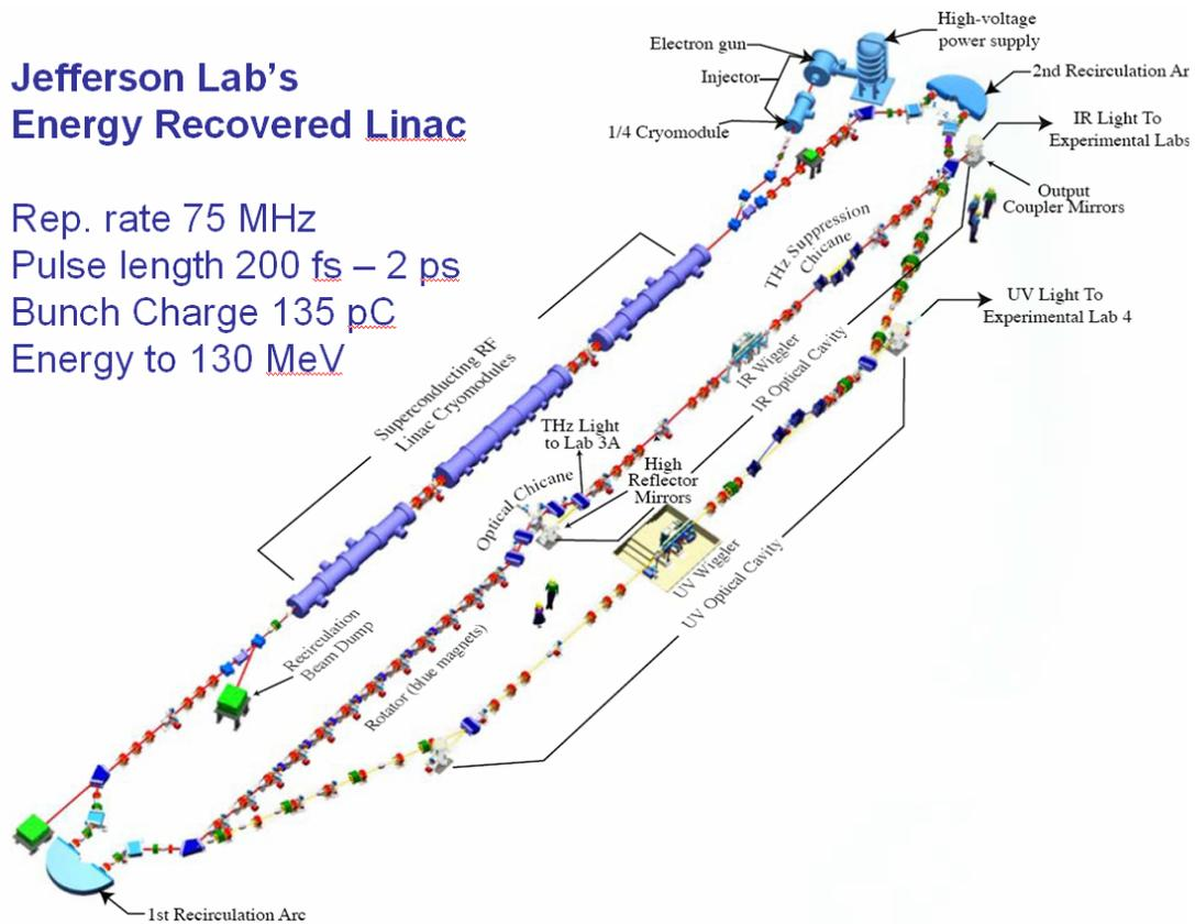
up to 75 MHz. CSR, or multiparticle coherently enhanced emission is produced by modulating this bunch in a Free Electron Laser cavity, and is also produced for wavelengths that are longer than twice the bunch length. With electron beam energies of 100 MeV, the electron beam energy is 1 MW. Therefore we energy recover the electrons in a return loop.
