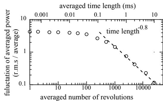
**Fig. 2.** Fluctuation of time-averaged power of CSR burst. The broken line is a guide which shows the dependence of period<sup>-0.8</sup>.
