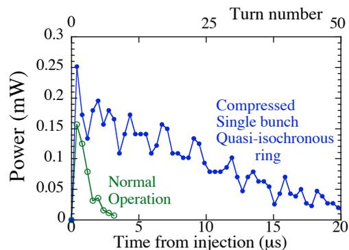
**Fig. 1.** The turn-by-turn coherent radiation power after injection. The line with open circles shows the power obtained with the parameters of normal operation, where there were three bunches in a pulse. The line with filled circles shows the power obtained from one compressed bunch in the quasi-isochronous ring. The bunch charge was about 0.02 nC/bunch in both cases.
